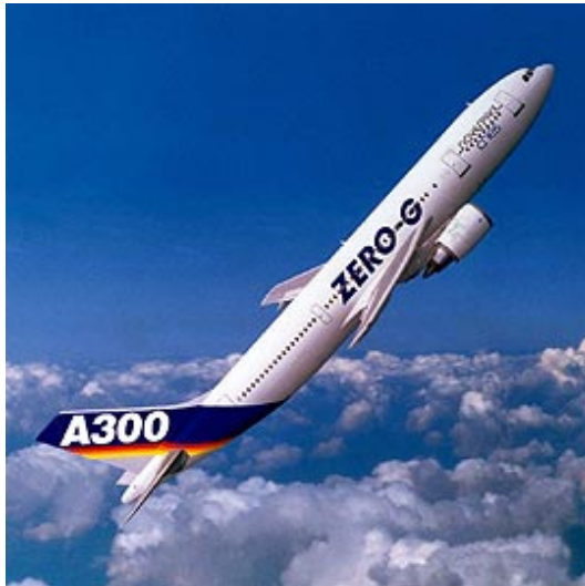
Experiments in zero gravity: The parabola flight with the Airbus A300 ZERO-G makes it possible. Figure: Novespace
